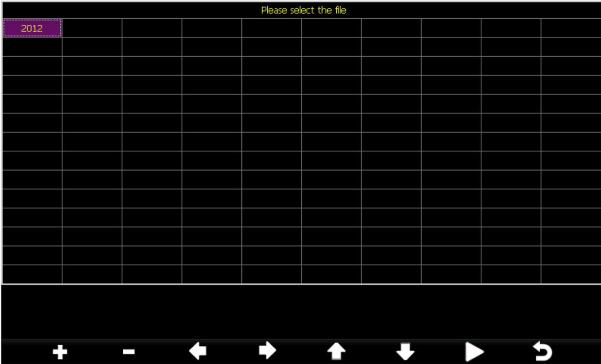
Press or key to select the history year file. Press key or key to confirm the selection. Press or to change the activated option field. Press key to start backup, press key again to stop the backup. Please insert TF card before start backup. The data save as excel format as default setting.
