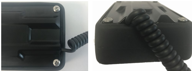
Figure 2. Sensor cable fed through slot
