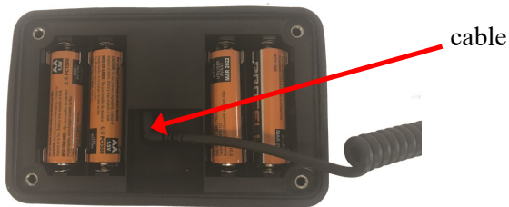
Figure 1. Sensor cable plugged into jack
