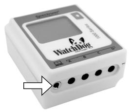
The **only time** you must have the WatchDog connected to the computer is during the launching and downloading of the data *logger*. After the logger has been launched, and/or downloaded, disconnect the logger and place it in the environment you wish to monitor.
