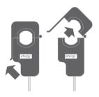
1. Push the release cap to open the sensor.
