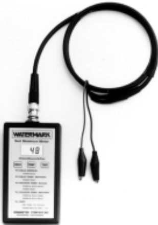
Watermark Electronic Meter (30-KTCD-NL)
