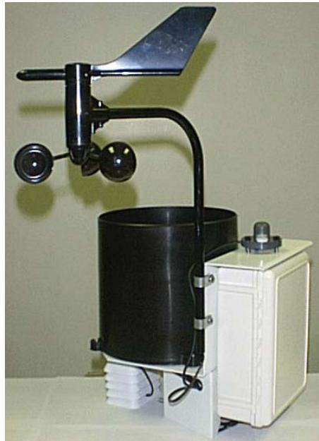
Apart from the anemometer, the WatchDog Weather Station comes fully assembled and ready to mount. The anemometer arm is attached to the enclosure back plate with two clamps. After positioning the arm, the screws should be tightened to secure it in place.
