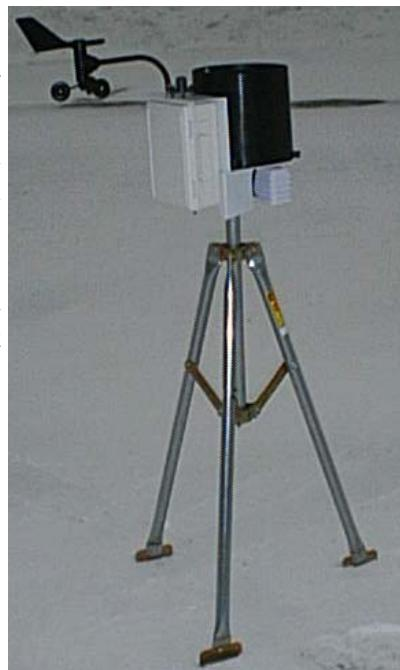
**Important:** Secure the external sensor wires to the mounting pole with a plastic tie. This will ensure that the sensor wires do not become disconnected while recording
