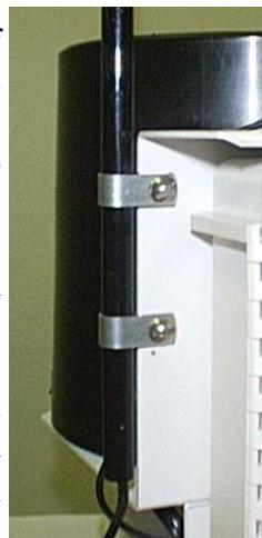
*Anemometer clamped to back plate (for visibility, black, rubber clamps not shown)*
