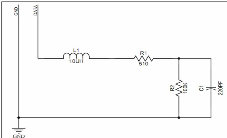
**NOTE:** This is a low impedance variant of the recommended SDI-12 Specification. This allows up to 62 sensors to be maintained on a bus.
