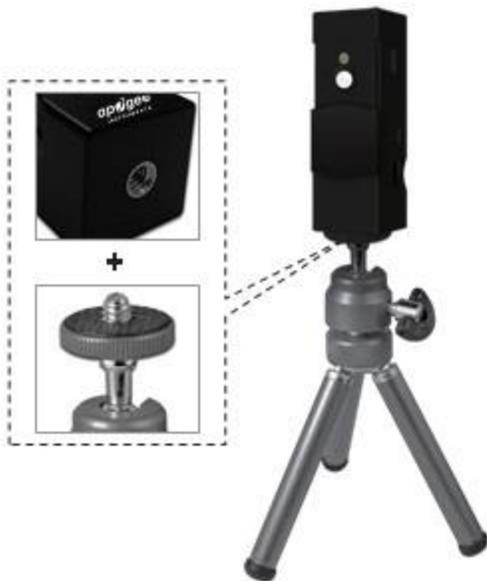
If you detach the lanyard screw on the bottom of the MS-100, it will expose a screw hole where you can attach a tripod for hands-free LED measurements.
