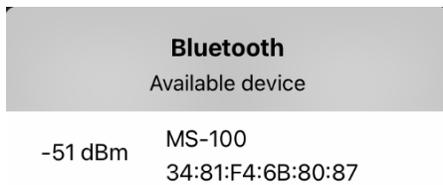
Select "Yes" when asked to reset the Bluetooth connection. Select the device that pops up under "Available Device." When the device has connected, it will show the "MS-100 Status."
