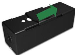
5. Slide the sensor cover down so that the sensor diffuser is visible again.
