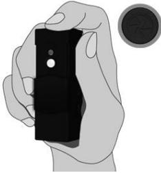
7. Hold the MS-100 as shown with the sensor facing toward the front, in the direction of a light source, and press the “measure” button on the top of the MS-100.
