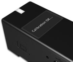
When Dark Calibration is complete, the screen will read “Calibration OK.”
