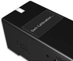
3. After the splash screen, a "Dark Calibration" label will display, indicating that a dark calibration is in progress.
