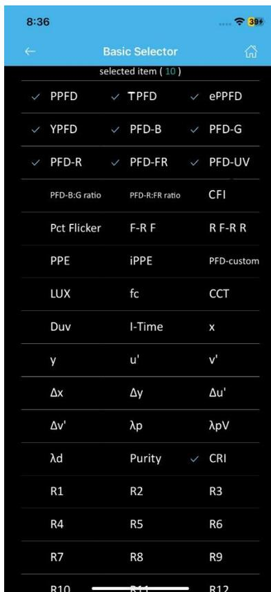
After selecting the gear icon, select the “Basic Selector” setting. By default, 10 measurements are displayed on the “Basic” screen, but you can select as many measurements as you need. Select the measurements you want and return to the “Basic” screen to capture data.
