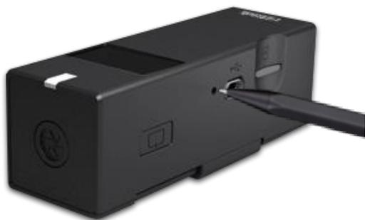
If for any reason you need to perform a system reset, you can use a pointer to press into the reset hole as shown.
