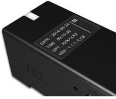
6. The first screen will display the date and time, optic number, and software version number. The battery level indicator is on the top right.
