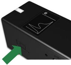
8. The measurement takes approximately 10 seconds to complete. The unit will beep to indicate completion. The screen will then show the wavelength spectrum. Press the On/Off button on the left side of the unit to go to the next measurement screen.
